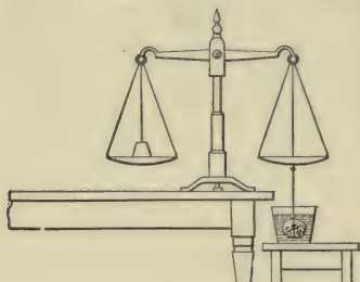
FIG. 2 Determining Specific Gravity by a Balance
